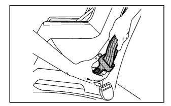
For third row seating positions, with cinching latch plates, tilt the latch plate to adjust the belt if needed.
